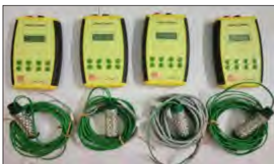
Soil moisture sensors with recording meters
